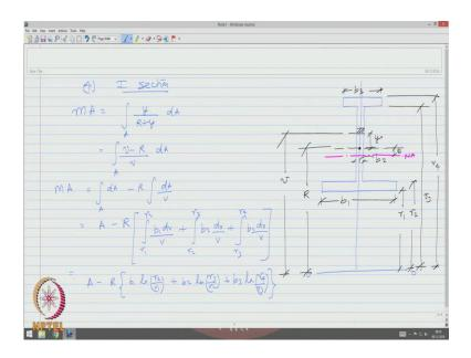
Let us take an I section; let us mark the plane o o; which contains a centre of curvature, let the dimensions be b 1, b 2 and b 3. We do not mark the thickness but we mark different radius from the centre of curvature or from the plane of centre of curvature as r 1, r 2, r 3 and of course this is r 4.
