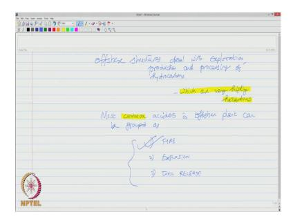
We all know that offshore structures deal with exploration, production and processing of hydrocarbons, which are very highly hazardous that is a very important statement which we must realize that hydrocarbons are very hazardous and most common accidents in offshore plant can be grouped as; one due to fire, two due to explosion and third due to toxic release.
