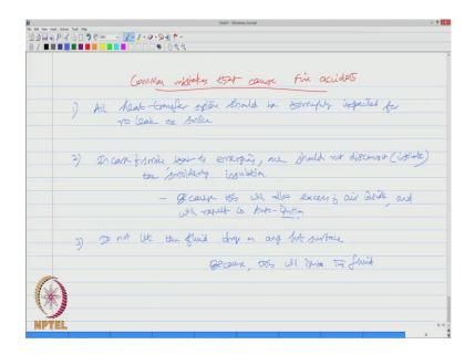
Let us ask a question; what are common mistakes people make that can cause fire accidents? 1. All heat transfer system should be thoroughly inspected for no leak or smoke that is a first practice which we would adopt, if violated can be one of the common mistake to cause fire accidents.
