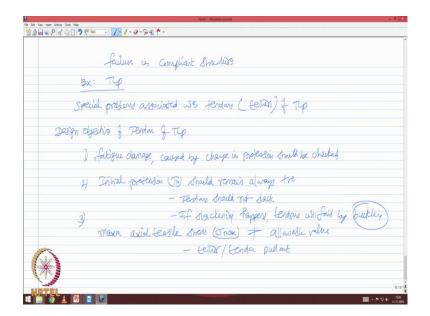
Very briefly we will talk about this; we will take an example as tension leg platform, there are some special problems associated with tendons or let say tethers of tension leg platform. What should be the design objective for designing a tendon of a TLP? Let us ask this question. What are the design objectives of tendon of a TLP? There are 3 objectives.
