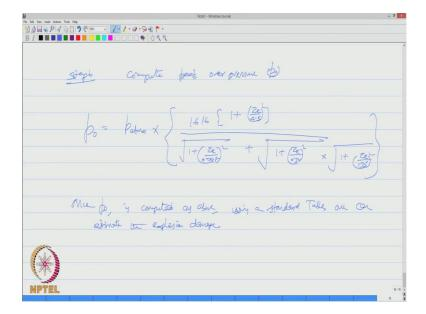
Then in step number 6, you are interested to estimate the damage so let us compute something called peak over pressure is P 0. P 0 can be given by this equation P at mas, multiplied by 1616, 1 plus Z e by 4.5 square root of 1 plus Z e by 0.048 square, plus root of 1 plus Z e by 0.32 the whole square multiplied by 1 plus Z e by 1.35 the whole square equation number. So, once over pressure P is computed as above using a standard table, one can estimate the explosion damage.
