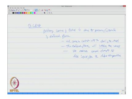
In explosion let us take up an important terminology which we discussed just now BLEVE primary cause of BLEVE is due to external flame or intervention of external flame, this external flame will come in contact with the shell of the vessel, this external flame will weaken the vessel, it reduces the vessel strength to hold liquid or gas at higher temperature.
