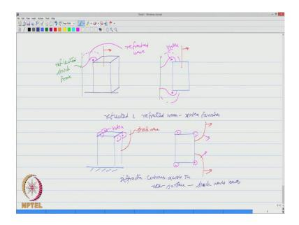
This is the original shock front this is reflected shock front. This reflection will also cause a refraction wave, this is what we call as refracted wave this refracted wave will induce vortices this will cause vortex whereas, the shock wave front this number here.
