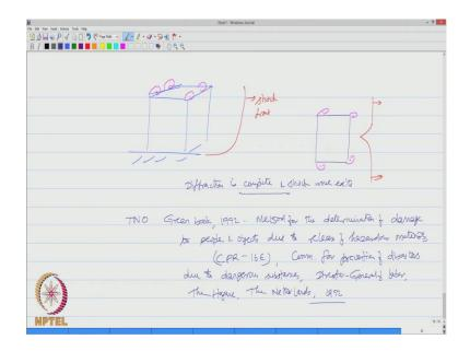
So, I should say here the diffraction continues across the near surface as the shock wave leaves the building then subsequently the vortices will be formed and the shock wave will completely leaving the building, it means the shock wave completely leaves and heat causes vortices. So, I should say here that the diffraction is complete and shock wave exceeds.
