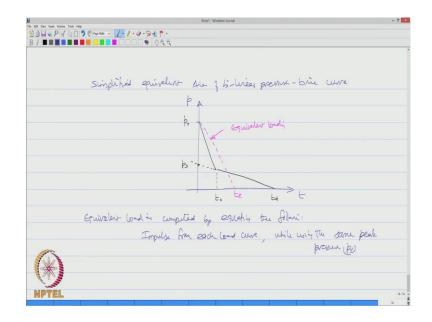
So, graphically a simplified equivalent triangle of bilinear pressure distribution curve, pressure time curve will explain this let say this t pressure versus time plot, this is the actual loading. So, this is my td and this is my tc, the reflected over pressure duration and extend is this is my p s and of course, this is my p r. The equivalent loading can be taken as, we call this as te this is the equivalent loads which has the component of p r and p s both as a modified measure.
