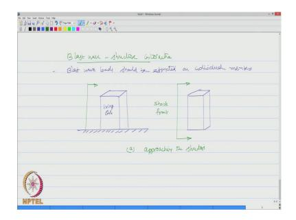
Let us talk about blast wave structure interaction. Blast wave loads should be estimated on individual members. The blast wave structure interaction can be explained interestingly by the graphical wave.
