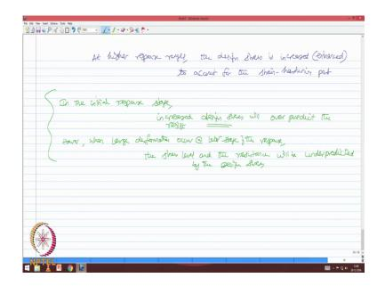
At higher response ranges, the design stress is increased I should say enhanced to account for the strain hardening part. Therefore in the initial response stage, the increased design stress will over predict the resistance because the design stresses are increased.
