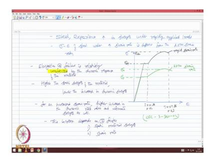
As we now understand, steel as a material, experiences increase in strength under rapidly applied loads. The stress strain behaviour of steel under increased strain rate is different from the ASTM strain rates as we talked in the last lecture. Just to capture back we said that the stress strain plot for two varieties of steel, let us say at rapid strain rate which can extend the strain, can go to till 0.07 to 0.23.
