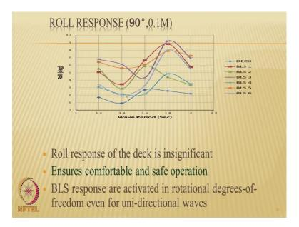
The role responses of the deck are far lesser than that of the buoyant legs, but still the response of the role degree happens in deck. It is because for uneven distribution of the responses of these legs happening at the sub structure.
