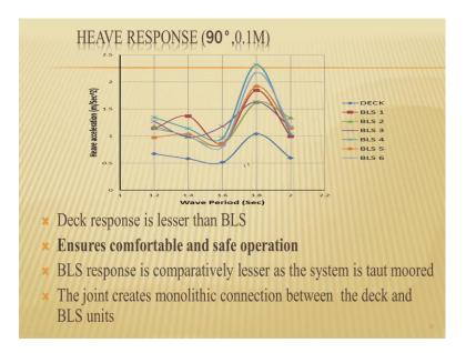
Similarly if you look at the heave response now; heave response of the deck is anyway lesser than that of the buoyant legs ensures comfortable and safe operation. And BLS response is comparatively lesser than the system; because the system is taut more. The joint creates of course a monolithic connectivity between the support system and the deck carefully by the design.
