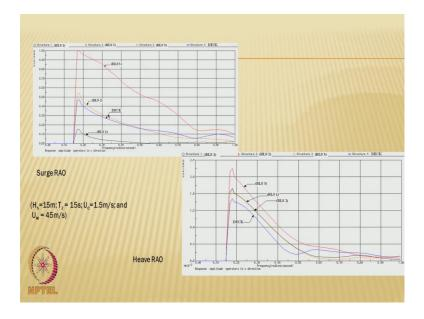
If you please play attention to the Rao plots that is response amplitude operator in the surge and heave degrees of freedom; one can see here the plots are done for frequency against the spectral density in the vertical axis, whereas four plots are done buoyant leg 1 set of legs 1, set of legs 2 and set of legs 3 and the deck.
