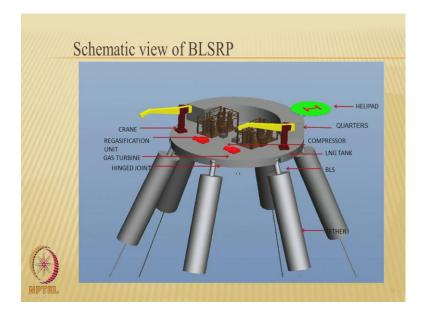
A typical schematic view of the structure is now shown on the slide. This consists of a deck which has all electro mechanic components. Usually the deck is circular because influence of the deck in terms of its area distribution or the mass distribution is more or less symmetric with respect to the cg. It has got a crane, helipad, living quarters, compressor units, regasification units, gas turbines etcetera.
