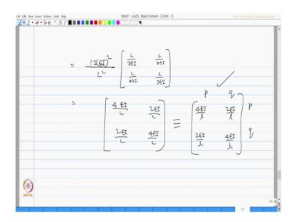
Which will amount to 12 E I square by L square of L by 3 E I; L by 3 E I; L by 6 E I; L by 6 E I; L by 6 E I which will be actually 4 E I by L. 2 E I by L. 2 E I by L and 4 E I by L.
