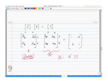
if I say delta j j delta j k delta k j and delta k k are the flexibility coefficients for j the and k th nodes; if I multiply this with p q and p q which are stiffness coefficients which is k p p, k p q, k q p and k q q, I will get an identity matrix which is 1, 0, 0, 1.
