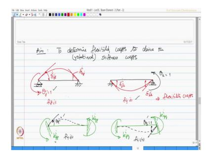
So, let us do that now. So, the job is to determine the flexibility coefficients to derive the rotational stiffness coefficients correct that is **our** task; now let us do that. So, let us take a beam which is simply supported; let us give unit rotation to this end.
