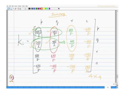
I am writing the full matrix of the ith member which is p, q, r, s which is p, q, r, s; the 4 values are 4 E I by L, 2 E I by L, 2 E I by L and 4 E I by L which we derive; just now I wrote that.
