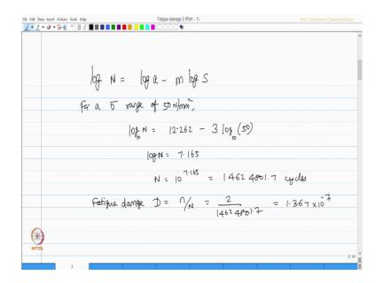
So, let us say we want to include the fatigue damage, we want to calculate the value n equation is log N is equal to log a minus m log S. Now for a stress range of 50 let us compute for a stress range of 50 Newton per mm square let us compute this so log n is equal to 12.262 that is my log a value minus 3 is my m value and log 50 there all log to the base 10 they are not Napier's logarithm that is log to the base 10 which gives me the value of log N as 7.165.
