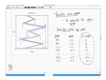
In the earlier example, the stress cycles were completely and readily given to you, but in this example the stress cycle is not given, but only the stress variation and time that is stress history is given. So, we need to conclude the stress cycle I can use rain flow count method this is one of the easy methods by which you compute the stress cycle say how we are doing it.
