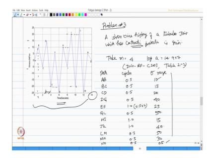
A stress time history, you can see here a stress time history time and stress time history of a tubular joint which has cathodic protection is given take M value as 4 and log a value for cathodic protection as 14.917 which is advised by DNV recommended practice C203 table 2 2 which we also dealt in the last example.
