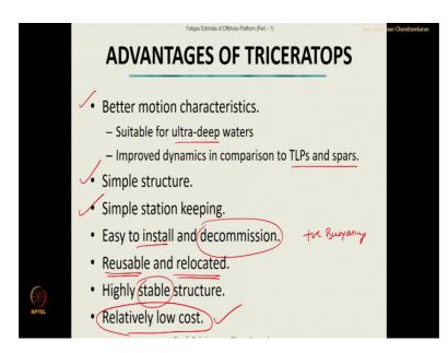
Triceratops have lot of structural advantages, it has got best better motion characteristics therefore, initial studies conducted in triceratops both numerically and experimentally confirm that they are highly suitable for deep waters and ultra deep waters.
