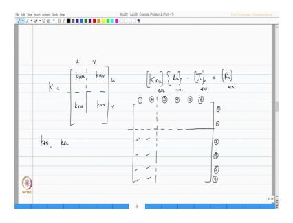
We said that K has got sub matrices K u u, K u r, K r u; K r r which we have partitioned the matrix. So, this is unrestrained restrained unrestrained restrained.
