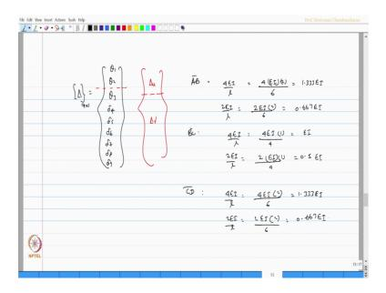
Having said this let us mark the displacement vector rotational and translational both which is going to be this is going to be 7 by 2 and this is going to be 7 by 7 total is 9. So, this is going to be a vector of 9 by one which will have theta 1, theta 2, then theta 3, delta 4, delta 5, 6, 7, 8 and 9 where I am going to do a partition at this level. So, this is also
