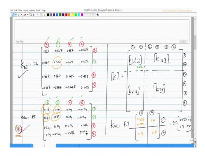
We have generated for example, 3 1 4 5; 3 1 4 5; we generated this stiffness matrix similarly for K B C 1 2 5 6; 1 2 5 6 generated, we partitioned the matrix and got K u u as 2 by 2 and we picked up K u u founded K u inverse and applied the joint loads computed the joint load vector partitioned the matrix for unrestrained restrained and unrestrained vector is picked up.
