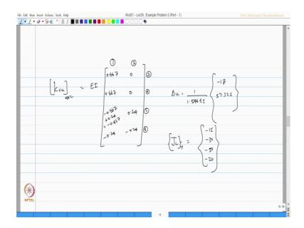
So, I fill up this matrix and I get K r u matrix 4 by 2 as below which is going to be E I of this is first row first column second column r. So, it was going to be 3, 4, 5 and 6. So, this value is 0.667; this value is 0.667 and this value is going to be minus 0.667 plus 0.24 which will be minus 0.427 in this is minus 0.24. So, this will be 0; this will be 0.24; this is minus 0.24.
