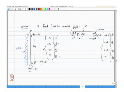
The next step is to find the fixed end moments caused because of the loads on each span of the member. Let us do one by one. Let us say span AB subjected to a uniform distributed load of 12 kilo Newton per meter and this distance is 6 meters; is or not. So, this will cause a moment as I am indicating here. So, this value will be 12 into 1 square by 12 which will be 36, this will also be 36, and this reaction will be 12 into 6 by 2 which will also 36 and 36.
