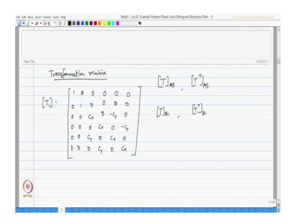
Transformation matrix T of any member I is actually given by it is 6 by 6 matrix 1, then 1 and 0 0 C x 0 C y, 0 then 0 0 0 C x 0 C y, then 0 0 minus C y 0 C x 0, then 0 0 0 minus C y 0 C x.
