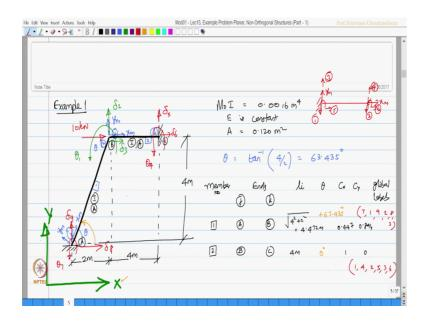
Let us take an example and solve this problem let us take example 1; this is my structural system which is fixed here as well as fixed here let us call this end as A, B and C; let us mark the dimensions of this structure. So, this is 2 meters. And let us say this is 4 meters; let the height of the frame be 4 meters. Now interestingly, this is my global axes and for every member the local axes is going to be different.
