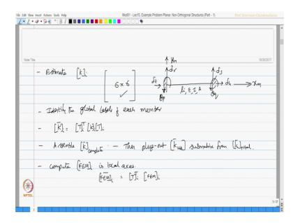
So, the next step is estimate the stiffness matrix of each member, we already have this equation with us derived in the last set of lectures; we know this is going to be a 6 by 6 matrix, we already have a fixed beam as our basic module, we know that this is going to be theta p theta q delta r delta s delta T and delta H where this is my x m axes this is my y m axes of the member the member has a length 1 I EI and A.
