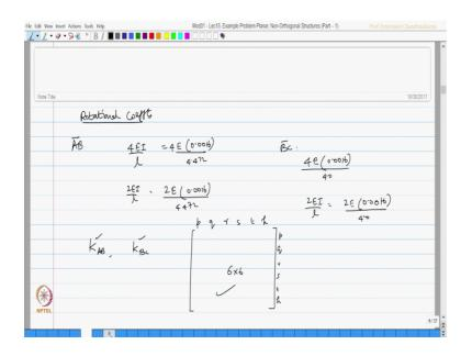
Let us compute the rotational coefficients because we need them for the stiffness matrix let us do it for the member AB you know it is going to be 4 EI by l which is going to be EI times 0.0016 by 4.472. Similarly 2 EI by l which is 2 times 0.0016 by 4.472; this is for the member AB, we can also do this for the member BC which is 4 times E 0.0016 by length of the member which is 4.0 and 2 EI by l which is 2 E 0.0016 by 4.0.
