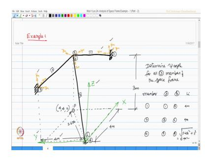
Now, I call this as my point P, I am choosing this point on x y m plane, I call this as my point P for the problem. So, the coordinates of this point with the reference axes system will be 4 comma, I can write it here 4 comma 4 comma 0 with reference to j-th end, it will be 0 comma 0 comma minus 3, correct; this end will be I write down that here coordinates of point P will be 4 comma 4 comma 0.
