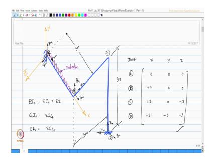
So, let us have a structural system as shown in the figure. Now, this is my structural system; let us mark the dimensions of this; this is 3 meters, let say this is also 3 meters and this height is also 3 meters; let us mark the nodes as A, B, C and D, let us say; it is subjected to some uniform distributed load as shown in the screen now the load intensity is 20 kilo Newton per meter.
