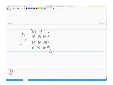
So, we all know that the transformation matrix t is simply given by cs of the member I, then 0 0 and 0. Similarly 0 cs 0 0 0 0 which we derived at is it not and 0 0 0 0 and cs which is 12 by 12.
