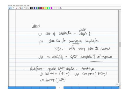
So, this geometric configuration, there are some issues; one cost of construction, two when you increase the water depth, two downtime for commissioning the platform; that is such platforms like GBS takes many years to construct. So, it takes lot of time to complete the construction and make the platform ready for oil exploration and, thirdly reusability of the platform after completion of oil source. So, this is an issue.
