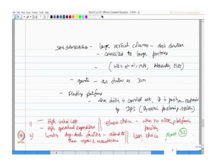
The moment you have compliant structures or floating structures, you will see that the displacements are much larger, which enables them to counteract the forces acting on them which is the concept in the design of these kinds of platforms. So, semisubmersibles have large vertical columns which are connected to large pontoons, columns actually support the deck structure.
