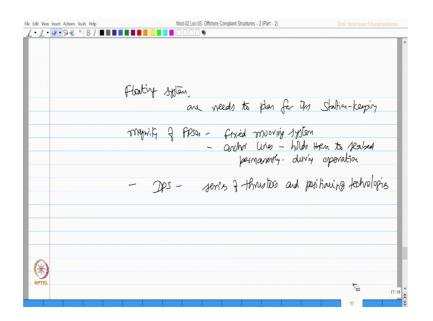
So as we all agree, now if you are deploying a floating system one needs to plan for its station keeping during, drilling and production. Majority of FPSOs, depend on fixed mooring system, they have anchor lines, which holds them down to the seabed permanently during operation.
