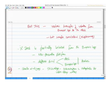
So friends, ball joints are designed to restrain transfer of rotations from buoyant legs to the deck, but transfers translational degrees or displacements. So, I should say now deck is partially isolated from the buoyant legs. So, that is the very important advantage which makes this platform as a new generation platform.
