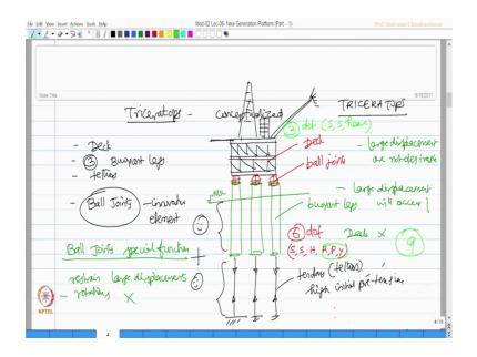
Having said this, a new system by name triceratops is conceptualized which consist of a deck 3 buoyant legs.
