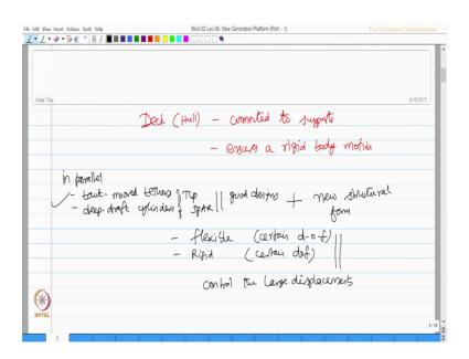
Deck or the Hull is connected to supporting system which ensures a rigid body motion. In parallel we also understand the taut moored tethers of TLP, and deep draft cylinders of spar are good designs. We agree that, because we saw the advantages of these points. So now, I want to capture this advantage into a new structural form.
