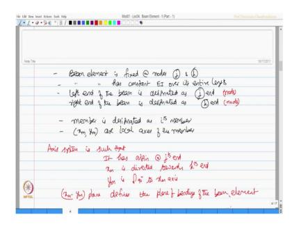
The considered beam element is fixed at nodes j and k, you can see here they are fixed at nodes j and k; has constant EI over its entire length. Left end of the beam is designated as j-th node. Right end of the beam is designated as k-th node; let us say j-th node and k-th node. Member is designated as i-th member xm ym are local axes of the member.
