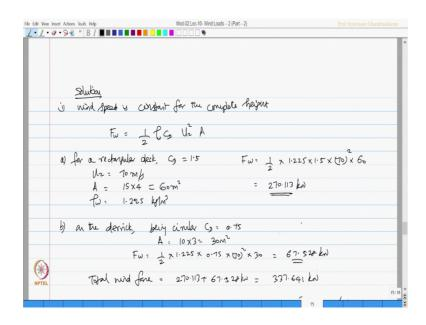
So, let us say solution, for the first case wind speed is constant for the complete height we know that force because of wind is given by half rho CD rho of wind CD U z square and the projected area.
