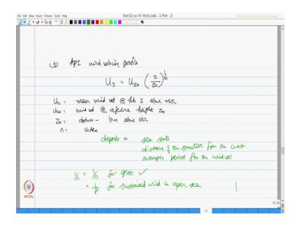
So, b using API wind velocity profile; we already given the governing equation for the spectrum AP wind velocity says U at any z will be given by U z 0 z by z 0, 1 by n where U z is the mean wind velocity at height z above the mean sea level U z 0 is wind velocity at reference height z 0. Z 0 is the datum which is generally 10 meters above the mean sea level and n actually is an index this index depends on sea state distance of the structure from the coast and averaging period for the wind.
