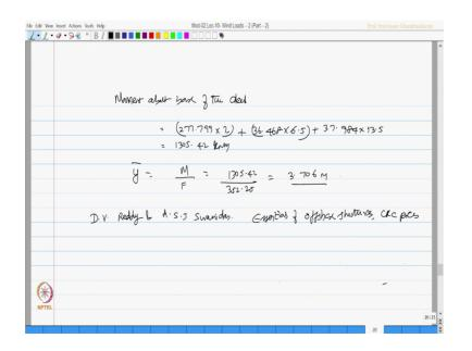
I want to now workout the moment, moment about base of the deck is going to be 277.799 into 2 that is a deck wall plus 36.468 into 6.5 plus 37.984 into 13.4 which gives me 1305.42 kilo Newton meter therefore, y bar cg is going to be M by F which is 1305.42 by 352.25 which is 3.706 meters.
