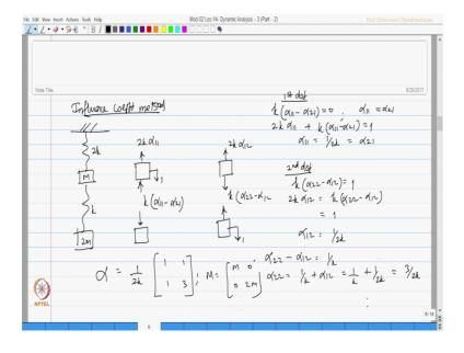
This is going to be m 2m this is 2 k and k, let us write the free body diagram so unit force. So, this is going to be 2 k of alpha 11 and this is going to be k of alpha 11 minus 21. Similarly for the second degree give unit force here. So, this is going to be k times of alpha 22 minus alpha 12 and this is going to be 2 k of alpha 12.
