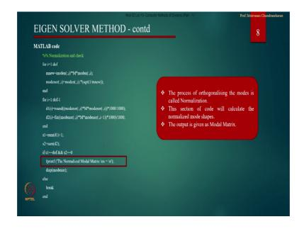
So, now normalization is being done and we get ultimately the normalized modal matrix with respect to mass. You can normalize the matrix modal matrix either with respect to mass or with respect to stiffness. So, in this case it is normalized with respect to mass.
