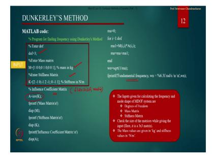
Then it calculates the influence coefficient matrix by inverting by inverting the stiffness matrix, inverse the standard subroutine in MATLAB. So, once k matrix is designated can invert the matrix to get influence coefficient. So, friends please remember influence coefficient matrix is nothing, but the flexibility matrix.
