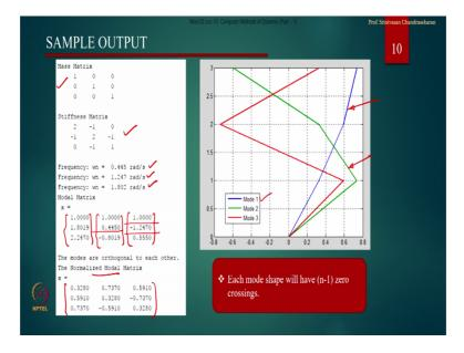
And there is a sample input mass matrix is been given stiffness matrix has been printed and it calculates all the 3 frequencies it calculates the corresponding omega 1 this is phi 1, omega 2 this is phi 2 and omega 3 this is phi 3.
