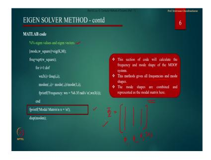
This method gives all frequencies and mode shapes the mode shapes are combined in a modal matrix is written here. So, in a model matrix of 3 by 3 because the 3 degree freedom system model, each column will refer to the each vector so this is phi 1, this column will be phi 2 and this column will be phi 3 together this matrix is called phi matrix or modal matrix.
