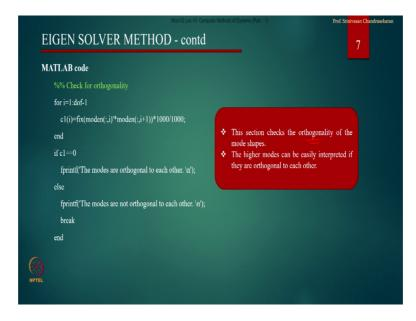
Then orthogonality condition is also checked for this given problem and if the modes are not orthogonal the modes are made orthogonal and one can find out that.
