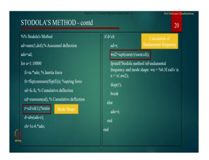
This is the mass value this is a k value once you do this the code actually identifies and computes accumulated deflection finds the mode shape plus iteration and then from the iterated value it picks up omega n square the fundamental frequency and then also picks up the mode shape. Let us see the sample output what we got from this code it is 0.445 and this is my vector. You can see this value closely agrees with what we have in influence coefficient method.
