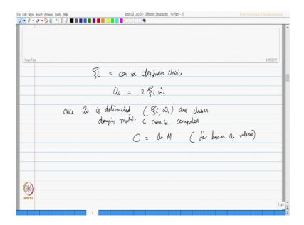
Once a 0 is determined it is a known value now because zeta i and the corresponding omega i are chosen damping matrix C can be computed which is C equals a 0 of m for known a 0 values.
