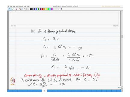
Similarly, for stiffness proportional damping Cn equals a 1 k, Cn is a 1 omega square m and zeta is equation number 4 zeta is Cn by 2 m omega n which is a 1, omega n square m n by 2 m n omega n which will give me zeta n as a 1 by 2 omega n. This says that the damping ratio zeta is directly proportional to natural frequency omega n.
