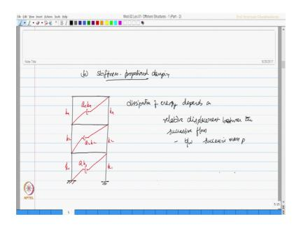
The next case could be a stiffness proportional damping. So, let us say we have again a multi story building we have each floor levels, each floor level will undergo relative displacement and now the damping model is expressed as a relative displacement between the floors.
