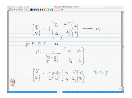
So, I can now say zeta i zeta j is actually equal to half of I am expressing this in a matrix form, I am expressing this relationship in a matrix form 1 by omega i omega i, 1 by omega j omega j of a 0 a 1. One can read this equation and similarly understand zeta i is equal to a 0 by 2 into 1 by omega i plus a 1 by 2 omega i which is as same as this.
