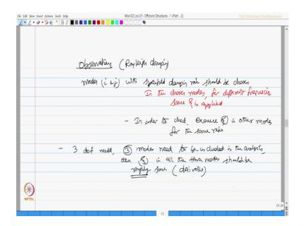
There are some observations on this condition some observations are - in applying this procedure of Rayleigh damping the modes i and j with specify damping ratio should be chosen. The condition is in the chosen modes for different frequencies same damping ratio is applied.
