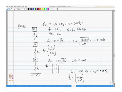
The example problem is let us say this is m 1, m 2 and m 3; this is k 1, k 2 and k 3. Let m 1 and m 2 and m 3 be a constant value which is 3500 kg, k 1 k 2 and k 3 be a constant value not constant let us take it like this k 2 is 1.5 k 1, and k 3 is 2 k 1, and k 1 is k which is 1500 kilonewton per meter let us say this data is given.
