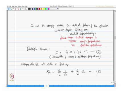
Rayleigh proposed damping which includes both C is going to be a 0 m plus a 1 k, therefore it is a combination of mass and stiffness proportional. In that case damping ratio at n-th mode is given by you know the damping ratio for stiffness proportional is equation 6.
