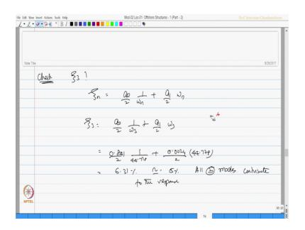
Now, I want to check what is my zeta 3, that is checking for the third mode zeta 3 I want to check. So, we know zeta n is a 0 by 2, 1 by omega n plus a 1 by 2 omega n. So, zeta 3 is a 0 by 2 omega 3 plus a 1 by 2 omega 3; a 0 we know is 841 by 2 by 44.778 plus a 1 is 0.0024 and omega 3 is 44.778 when you estimated this I get this as 6.31 percent which is very close to 5 percent hence we can say all 3 modes contribute to the response.
