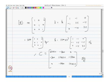
Summing them all we get C matrix as 6543.5 minus 3600 0, minus 3600, 0 11943.5 minus 540, minus 5400 15543.5 in so many Newton second per meter because k matrix is in Newton per meter mass matrices is in kg, C matrix is this.
