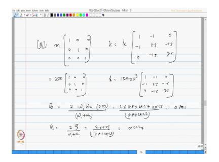
So, the mass matrix is now known to me which is m times of 1 0 0, 0 1 0, 0 0 1. From the equation of motion by force Newton's force method I can also find the k matrix I leave this is an homework to you, k will be actually equal to 1 minus 1 0, minus 1 2.5 minus 1.5 and 0 minus 1.5 and 3.5 that is my k matrix now. So, m matrix can also be said as 3500, so much 1 0 0, 0 1 0, 0 0 1 in kg and k matrix can be now said as 1500 into 10 power 3 of 1 minus 1 0, minus 1 2.5 minus 1.5, 0 minus 1.5 3.5.
