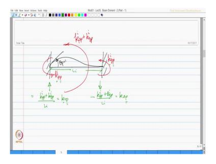
I have an element with both ends fixed; we have given unit rotation at the end p. So, now to control this, this will induce a moment which will be equal to k pp. This will also cause another moment which is k qp of the i-th element.
