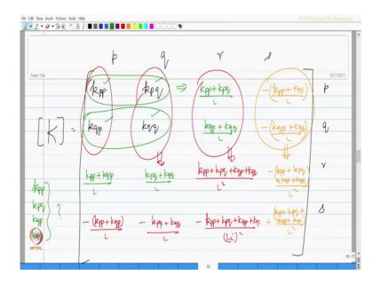
So, I can now make a matrix saying that the k matrix which will be p q r and s; p q r and s. This is k pp, this is k pq, and this is k qp, this is k qq; row first and column next. I evaluate only this four, remaining are derivable very simply this is k pp plus k pq by L
