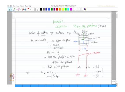
If you look at the problem formulation for analyzing a TLP, essentially TLP consists of a deck which will have all tops I details as drilling derrick, living quarters, flare boom etcetera which will be supported by the column members and pontoon members.
