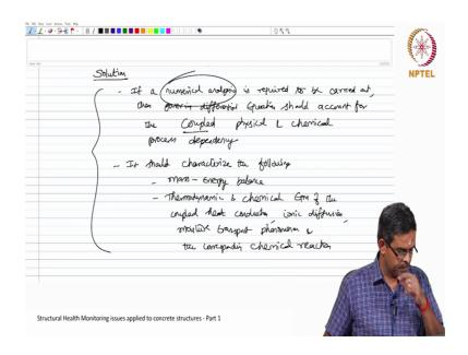
The question comes what is the solution for this problem, if a numerical analysis required to be carried out, then the governing differential equation, why differential? Because it is time variant as well as space variant. So, governing differential equation should account for the coupled physical and chemical process dependency. It should characterize the following.
