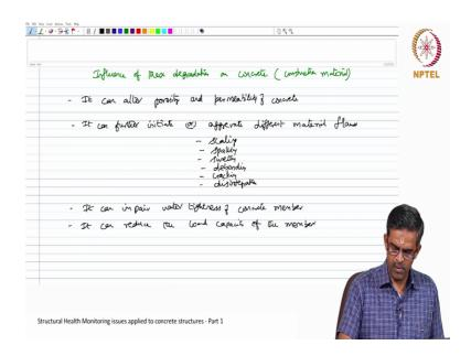
So, influence of these degradation on concrete as a construction material are as follows. These degradations can alter porosity and permeability of concrete. It can further initiate or aggravate different material flaws such as scaling, spalling, swelling, debonding, cracking, disintegration of concrete, etcetera.
