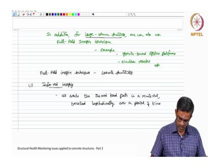
In addition, for large volume structures, one can also use full-field imaging technique. Example can be gravity based platforms offshore platforms, nuclear reactors etcetera.
