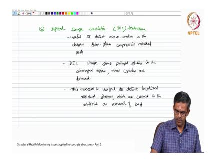
The third method applicable successfully to concrete structures is digital image correlation DIC technique. This is useful to detect micro cracking in the chopped let us say fiberglass compressive molded parts.
