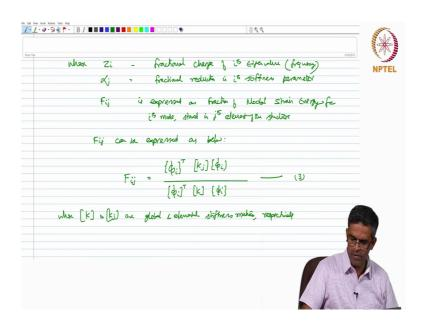
Where Z i indicates the fractional change of ith eigenvalue that is, frequency. Alpha j indicates the fractional reduction in i-th stiffness parameter. And F i j is expressed as fraction of modal strain energy for the i-th mode, stored in j-th element of the structure. F i j can be expressed as below. F i j yes phi i transpose K j phi i divided by phi i transpose K of phi i, where K and K j are global and elemental stiffness matrix, respectively.
