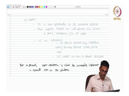
On the other hand, if a compare visual inspection method, it is actually done periodically or at schedule intervals. These periods of inspection intervals or well planned and becomes a part of the technical maintenance of the structural system. More or less visual inspection are contractual.
