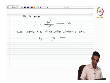
This is given by Z i is equal to del omega i square by omega i square. Further, sensitivity of the ith modal stiffness of jth element is given by F ij which is K ij by K i.
