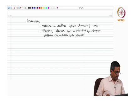
Let us say for example, reduction in stiffness intuits formation of cracks. Therefore, damage can be identified by change in stiffness characteristics of the structure. Let us see different methods and now, start comparing and contrasting the method within itself.
