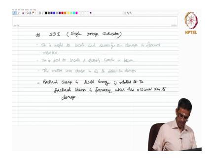
The next available method is b which is SDI which is called Single Damage Indicator. This method is useful to locate and quantify the damage in flexural members. Essentially, this method is good to locate and quantify cracks in beams to be very specific.
