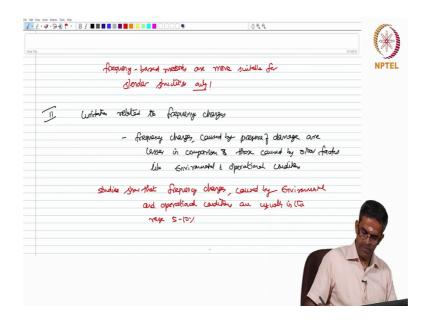
Therefore frequency based methods are more suitable for slender structures, I should say only with an emphasis.
