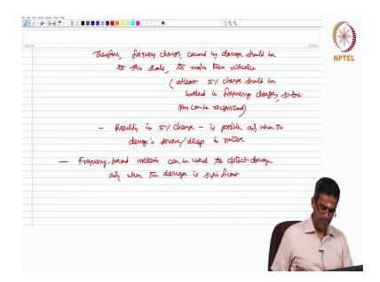
Therefore, frequency changes caused by damage should be to this scale to make them noticeable. It means at least 5 percent change should be invoked in frequency changes so, that they can be recognized.
