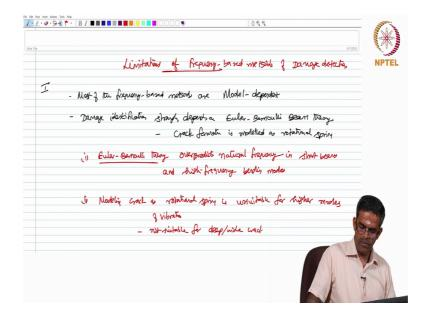
So, now let us see; what are the limitations in general of frequency based methods of damage detection. First most of the frequency based methods we have highlighted 3 of them or model dependent, damage identification strongly depends on Euler Bernoulli Beam Theory. In this beam theory crack formation is modeled as rotational spring.
