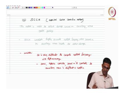
The next method in frequency based damage detection is SCCM, which is Spectral Center Correction Method. This method is useful, to detect damage based on auxiliary, mass spatial probing. Actually SCCM correlates highly accurate natural frequency value based on the auxiliary mass location to detect damage.
