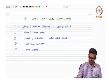
So, far we have seen method using change of frequency to damage detection, that is the first method we have seen, the second method is change in mode shape, the third analysis of mode shape using modern signal processing, the fourth method is mode shape curvature, which are essentially derivatives of the mode shape and the fifth method is what we are now seeing is the model strain energy method.
