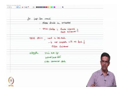
Now, when you go for long term monitoring sensor should be embedded in this structure. So therefore, here the main channels comes is human intervention and hash environment. Further, the IEEE protocol 802.11, which is used in the lab scale is not compatible with all kinds of ocean environment. So, there are alternatives. Alternatives could be voice over IP, broadband data, and video communication services.
