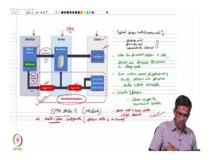
Now, the Structural Health Monitoring System what we have discussed also has an additional advantage, which is the alert monitoring system. So, look at the figure here this is actually the layout of SHM design to which we are discussing for the lab scale, that typical sensor node what we have here is a combination of is a combination of sensing unit, processing unit, and communication channel. It contains all.
