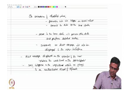
So on exceedance of the threshold value, the processing unit will trigger the processing unit will trigger an email alert and subsequently also transmits the data to the base station. Now server in the base station will process this data and performs detailed analysis, subsequently an alert message will also be displayed in the user interface. Now there are many advantages of this the alert message displayed on the monitor of the user of the user reduces the workload on the administrator ok.
