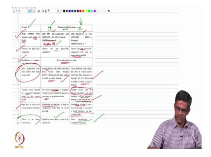
Let us compare them and see how was the result, wired sensors had 393B04 PCB module and spider 8 data acquisition system whereas, wireless system had PIC, PIC microcontroller and ADXL 335 802 15.4 Protocol for system 1, this is system 1 and system 2 had raspberry pi board with MPU 6050 802.11 x protocol for system 2. This we have explained.
