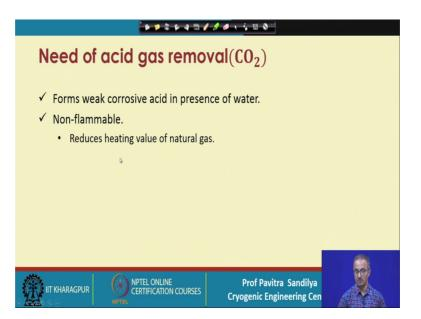
Why we need to remove carbon dioxide? Because it again forms weak corrosive acid in presence of water like H 2 S and it is non flammable and that is how it reduces the heating value of the natural gas.
