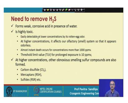
Now, why do we need to remove hydrogen sulfide? Because it forms weak corrosive acid in presence of water it is very toxic. And though it can be detected easily at low concentrations because it gives a rotten egg smell, but at high concentration it numbs our olfactory system. Olfactory means that our smelling system is affected so that we cannot smell it that at high concentration, but and when we cannot smell it, but it is going inside
