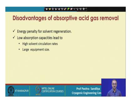
However, the disadvantages are that we have to spend energy for the solvent regeneration and they have low absorption capacity that that leads to high solvent circulation rate and large equipment size.
