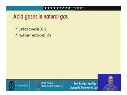
So first, let us see what are the acid gases in natural gas? They are carbon dioxide and hydrogen sulfide.
