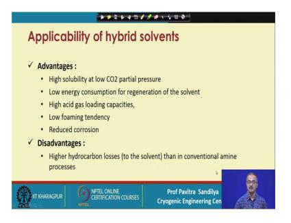
And these are the applicability of solvents and advantages are that; there are high solubility at low carbon dioxide partial pressure, they are low energy consumption for regenerating the solvent. And they have very high capacity to remove the acid gases, they do not form much and they have very low corrosion tendency. These are the advantage are that there will be high hydrocarbon loss to the solvent than the conventional amine processes.
