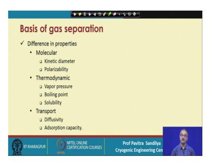
Now, there are various basis of the gas separation; in this case either we go a molecular properties like kinetic diameter, polarizability; then thermodynamic properties like vapor pressure, boiling point, solubility, then transport property like diffusivity, adsorption property. So, all these properties will dictate that which type of method we have to adopt for a given application.
