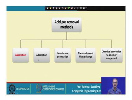
So, here are the various methods absorption, adsorption, membrane permeation, thermodynamic phase change and chemical conversion to another compound and in this particular lecture we shall be focusing on absorption.
