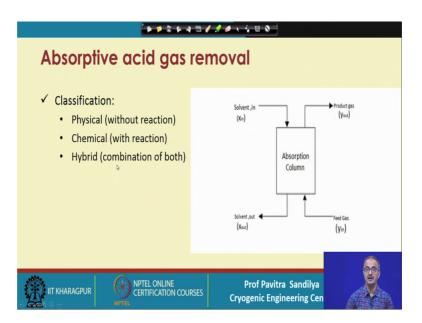
Now let us come to the absorptive acid gas removal; here we find from this diagram a typical arrangement to remove these gases by absorption. Here we have an absorption column and we are feeding the gas from the bottom and the solvent some solvent is fed from the top, it comes down and it moves up and they are mixing counter currently in this particular column.
