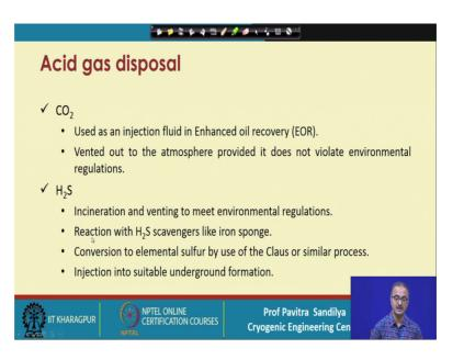
Now, when we talk of this acid gas disposal how we can dispose of carbon dioxide? That we can dispose of dispose it by injecting in an enhanced oil recovery system. And this is the method to recover any residual petroleum oil in which are entrapped in the rock formation in the sediment.
